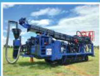
RC Drilling RIG
